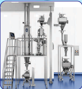
CONTAINMENT GRANULATION SYSTEM
